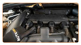
Detach the connector from the ignition coil.
