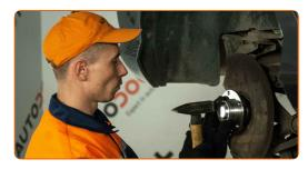
Install the brake disc.
