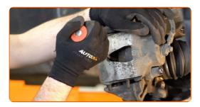
Remove the brake caliper.
