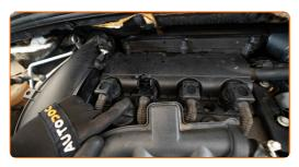
$\Lambda$  Detach the connector from the ignition coil.
