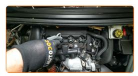
6 Unscrew the spark plugs. Use the 12-point spark plug socket #14.
