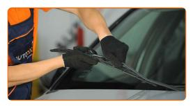
Remove the blade from the wiper arm.
