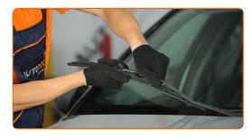
Remove the blade from the wiper arm.
