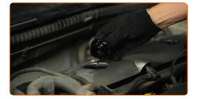
Tighten the oil filler cap.
