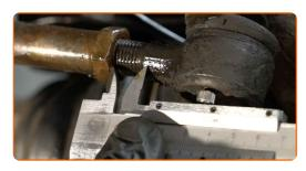
Loosen the lock nut securing the tie rod end to the tie rod. Use a combination spanner #16. Use a combination spanner #22.
