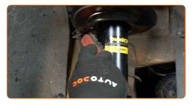
Unscrew the fastener connecting the stabilizer link to the shock strut. Use a drive socket #17. Use a ratchet wrench.
