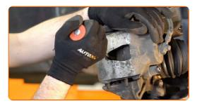
Remove the brake caliper.
