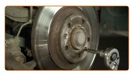
16 Remove the brake disc.
