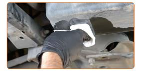
Screw in the new drainage plug and tighten it. Use HEX No.H6. Use a torque wrench. Tighten it to 30 Nm torque.
