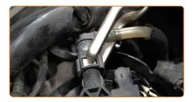
Replacement: fuel filter – PEUGEOT 407 SW Box Body / Estate (6E\_). Tip:
