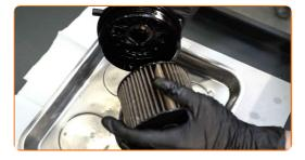
Clean the fuel filter housing and the cover. Use all-purpose cleaning spray.
