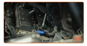
Plug in the ignition coil connector.
