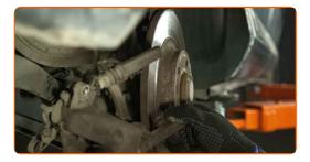
Tighten the brake caliper bracket. Use Torx T55. Use a torque wrench. Tighten it to 108 Nm torque.
