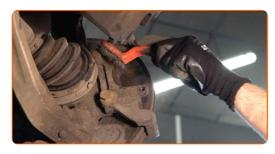
Unscrew the caliper bracket fastening. Use Torx T55. Use a ratchet wrench.
