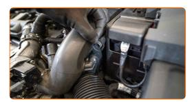
Connect the vacuum sensor. Squeeze the clamp with combination pliers and connect the vacuum valve hose.
