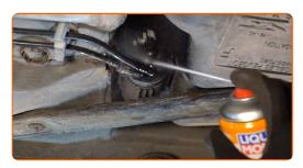
Remove the fuel lines from the car body.
