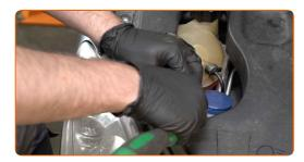
Remove the coolant reservoir cap.
