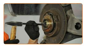
Unscrew the wheel hub axle nut. Use a drive socket #41. Use a ratchet wrench.
