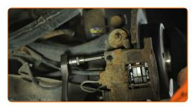
Use a drive socket #16. Use a torque wrench. Observe the recommended tightening torque.
