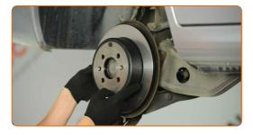
Remove the hub bearing protection cap. Use a crowbar. Use a rubber mallet.
