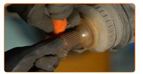
55 56 Install the steering knuckle on the CV axle.
