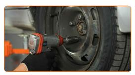
Lower the car and working in a cross order, tighten the wheel bolts. Use wheel impact socket #19. Use a torque wrench. Tighten it to 90 nm torque.
