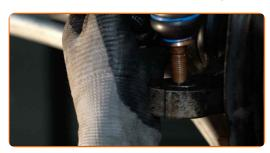
Tighten the fastening nut connecting the tie rod end to the steering knuckle. Use a drive socket #17. Use a torque wrench. Tighten it to 35 nm torque.
