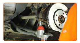
Tighten the tie rod end locknut. Use a combination spanner #24. Use a torque wrench. Tighten it to 60 nm torque.
