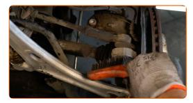
Unscrew the end fastening nut to the steering knuckle. Use a drive socket #16. Use a ratchet wrench.
