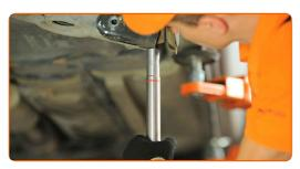
Tighten the fastener connecting the control arm to the rear knuckle. Use a combination spanner #21. Use a drive socket #21. Use a torque wrench. Tighten it to 95 Nm torque.
