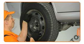
6 Support the rear control arm. Use a hydraulic transmission jack.
