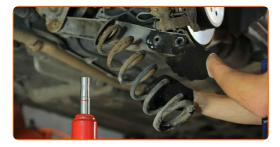
Remove the rubber spring spacer.
