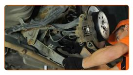
Support the rear control arm. Use a hydraulic transmission jack.
