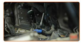
Plug in the ignition coil connector.
