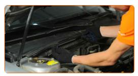
Remove the filter element from the filter housing. Use a flat screwdriver.
