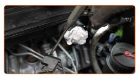
Unscrew the glow plugs. Use the spark plug socket #12. Use a torque wrench.
