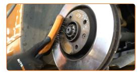
Unscrew the brake disc fasteners. Use Torx T30. Use a ratchet wrench.
