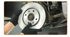
Tighten the brake disc fasteners. Use a Phillips screwdriver. Use Torx T30. Use a torque wrench. Tighten it to 10 Nm torque.
