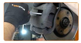
Remove the brake caliper. Use a crowbar.
