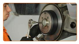
14 Remove the brake disc.
