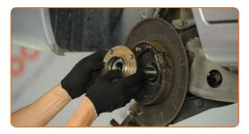
Clean the wheel hub mounting seat. Use all-purpose cleaning spray.
