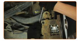
Unscrew the brake caliper fasteners. Use HEX No.H7.
