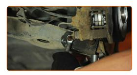
9 Remove the fastening bolt.
