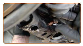
Tighten the lower fastener of the shock absorber. Use a combination spanner #18. Use a drive socket #18. Use a torque wrench. Tighten it to 75 Nm torque.
