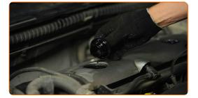
Tighten the oil filler cap.
