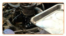
Detach the old filter cartridge from the filter housing cover. Use a crowbar.
