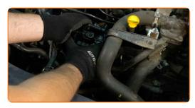
Attach the fuel pressure sensor connector.
