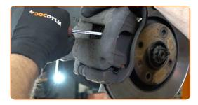
Remove the brake caliper. Use a crowbar.
