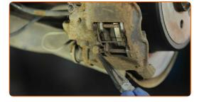
Remove the brake pads retaining clips. Use a pin punch. Use a hammer.
