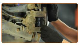
Install the brake pads retaining clips. Use a crowbar. Use a hammer.
