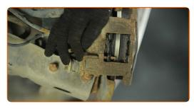
Install the retaining springs of the brake pads. Use round-nose pliers.
