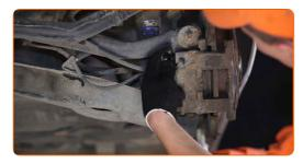
Unscrew the brake caliper fasteners. Use HEX No.H7. Use a drive socket #16. Use a ratchet wrench.
