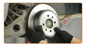
Tighten the brake disc fasteners. Use Torx T30. Use a torque wrench. Tighten it to 10 Nm torque.
