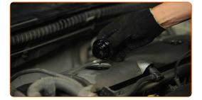
Tighten the oil filler cap.
