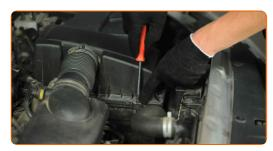
A Remove the air filter cover.
