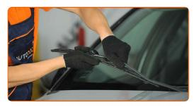
Remove the blade from the wiper arm.
