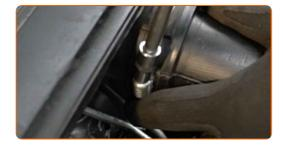
Connect the earth cable terminal to the battery.
