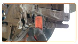
Unscrew the brake caliper fastening. Use a combination spanner #19. Use a drive socket #13. Use a ratchet wrench.
