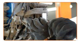
Remove the brake caliper.
