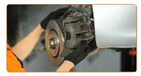
73 Treat the brake caliper bracket fasteners. Use a sealant.
