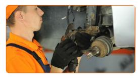
Remove the support from under the steering knuckle.
