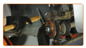
Install the ABS sensor on the steering knuckle and secure it. Use a drive socket #10. Use a ratchet wrench.
