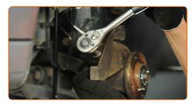
62 Connect the tie rod end to the steering knuckle.
