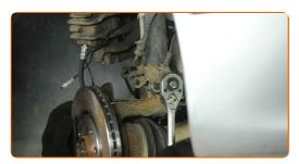
Remove the bracket from the suspension strut.
