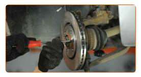
18 Remove the brake disc.
