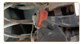
Release the parking brake cable. Use water pump pliers. Use pliers. Use a crowbar.
