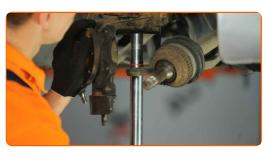
Fix the shock absorber strut on the steering knuckle. Use a hammer.
