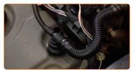
Remove the crankcase ventilation hoses.
