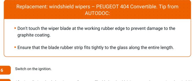
After installation check the wipers performance. The blades shouldn't intersect or bump against the windshield seal.
