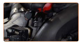
Unscrew the oil filler plug. Insert the funnel.
