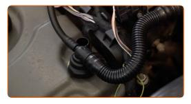
Remove the crankcase ventilation hoses.
