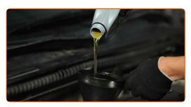
Replacement: engine oil and filter – PEUGEOT 309 II Hatchback. Tip from AUTODOC experts:
