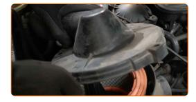
Remove the filter element from the filter housing.
