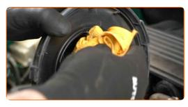
Insert a new filter element into the filter housing. Make sure that the filter edge fits tight to the housing.
