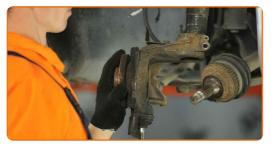
Unscrew the fastener connecting the ABS sensor to the steering knuckle. Use a drive socket #10. Use a ratchet wrench.
