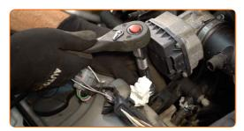
Replacement: spark plugs – PEUGEOT 309 Box Body / Hatchback (10S, 3S).
