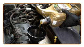
Replacement: engine oil and filter – PEUGEOT 308 SW I Box Body / Estate (4E\_). Tip from AUTODOC:
