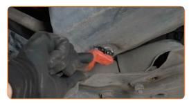
Unscrew the drain plug. Use HEX No.H6. Use a ratchet wrench.
