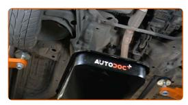
6 Clean the area of the oil pan drainage hole. Use a wire brush. Use all-purpose cleaning spray.
