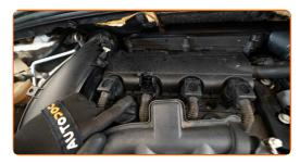
Detach the connector from the ignition coil.
