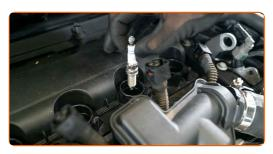
Screw new spark plugs and tighten them. Use the 12-point spark plug socket #14. Use a torque wrench. Tighten it to 23 nm torque.
