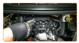
Unscrew the spark plugs. Use the 12-point spark plug socket #14.
